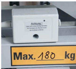
Deactivation of height-adjustment mechanism by means of a safety box
