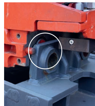
Tool clamped by engagement pins, but not properly locked
