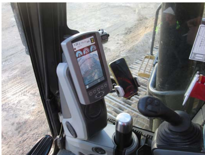
Figure 3: Small monitor, temporarily switched on, which can be used to display machine data and status information
